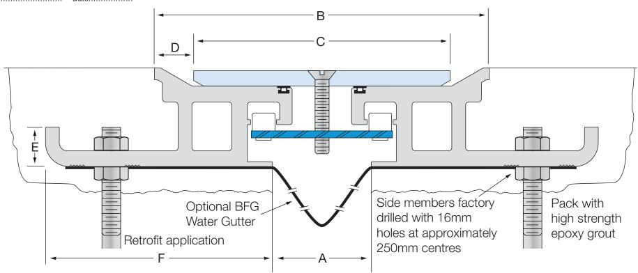
Cover plate loadings indicated are calculated under vehicular conditions, based on a 150mm diameter load circle, with a maximum allowable deflection of 3.2mm when calculated in the nominal indicated joint width position.
