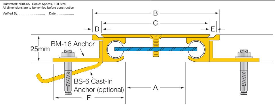
All anchors are supplied welded to the side members at approximately 475mm centres. BM-16 anchors are supplied factory drilled with 10mm holes at approximately 475mm centres
