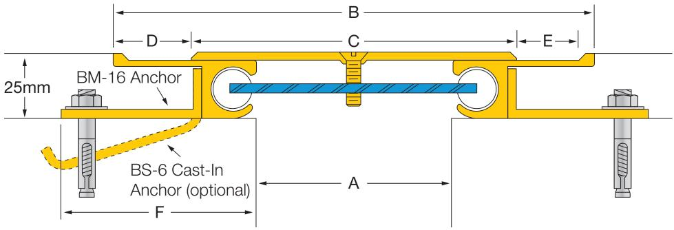
All anchors are supplied welded to the side members at approximately 475mm centres. BM-16 anchors are supplied factory drilled with 10mm holes at approximately 475mm centres
