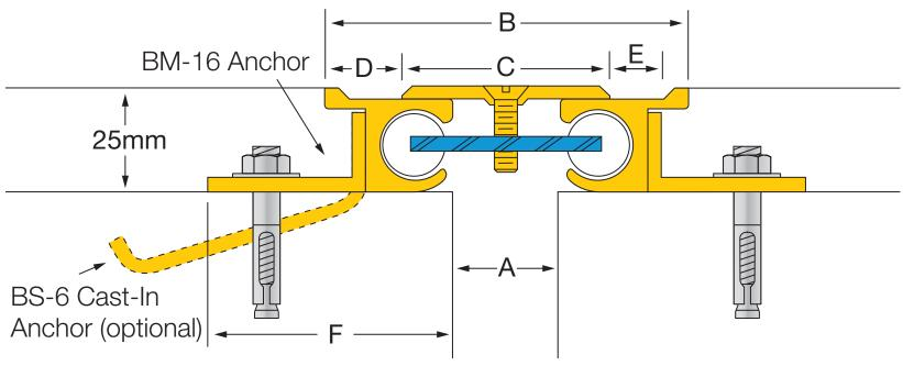
All anchors are supplied welded to the side members at approximately 475mm centres. BM-16 anchors are supplied factory drilled with 10mm holes at approximately 475mm centres
