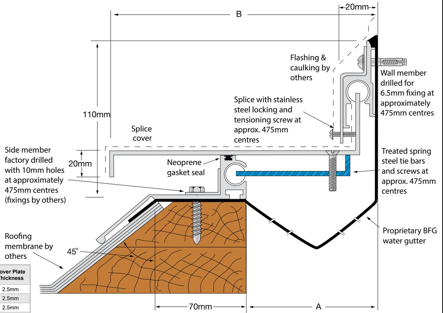
\* Tensioning tie bar for joint width larger than 150mm
